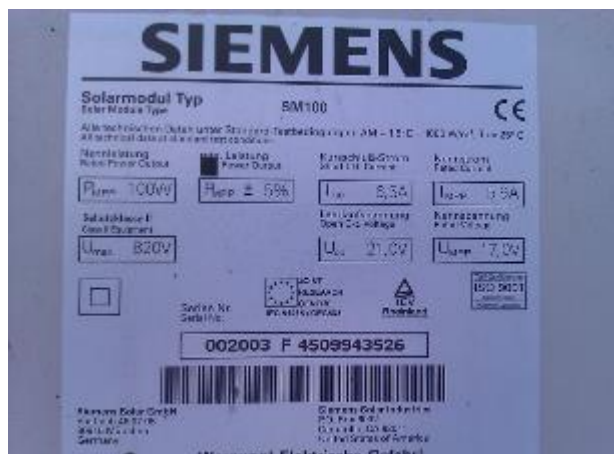
Fig 64 Solar Plate Specifications
